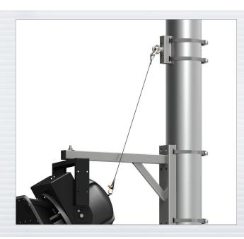
When the pole or column does not offer an adequate way to attach safety cables, specify the PM-Safety-6Down and corresponding band kit. This mount provides a structural method for anchoring safety cables.
